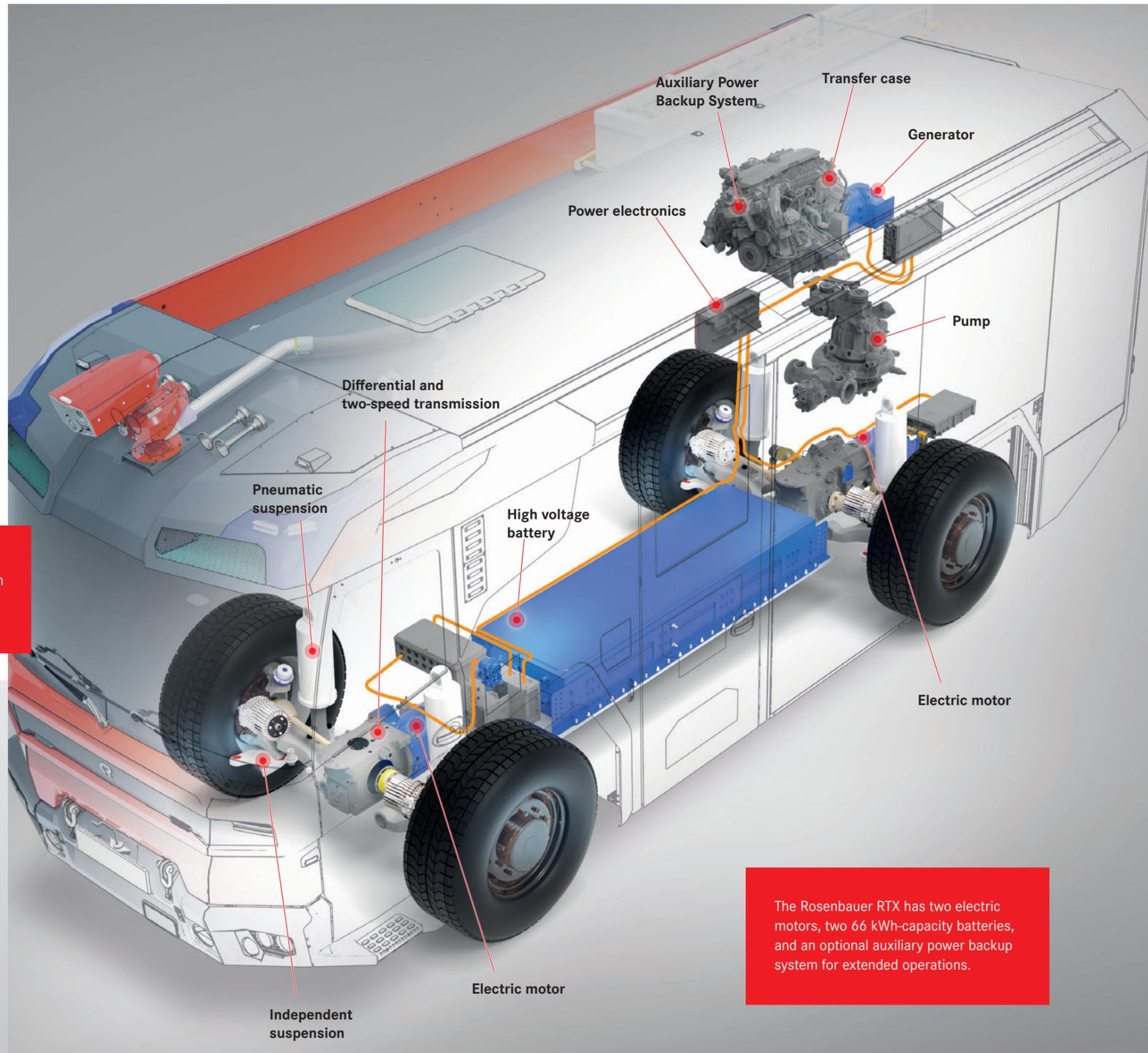
The Rosenbauer RTX has two electric motors, two 66 kWh-capacity batteries, and an optional auxiliary power backup system for extended operations.
